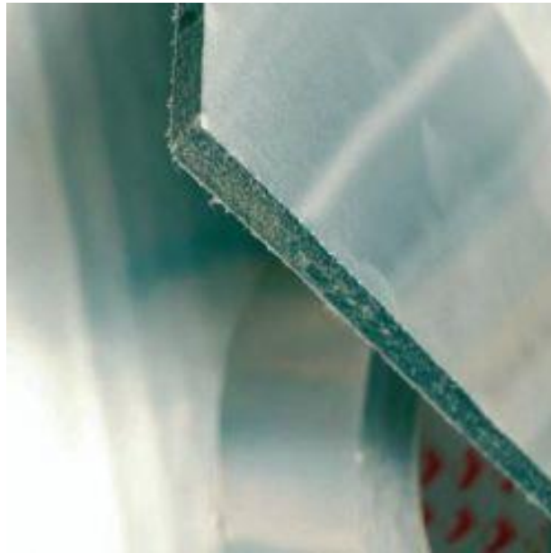
FIGURE 2. PICTURE OF ENERGAIN® PCM PANEL. THE PHASE CHANGE MATERIAL IS SANDWICHED BETWEEN FOIL MATERIAL AND EDGES ARE SEALED WITH FOIL TAPE.
