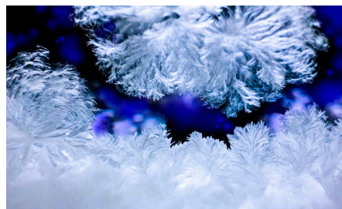
Microscopic image of BioPCM during a phase change transition
