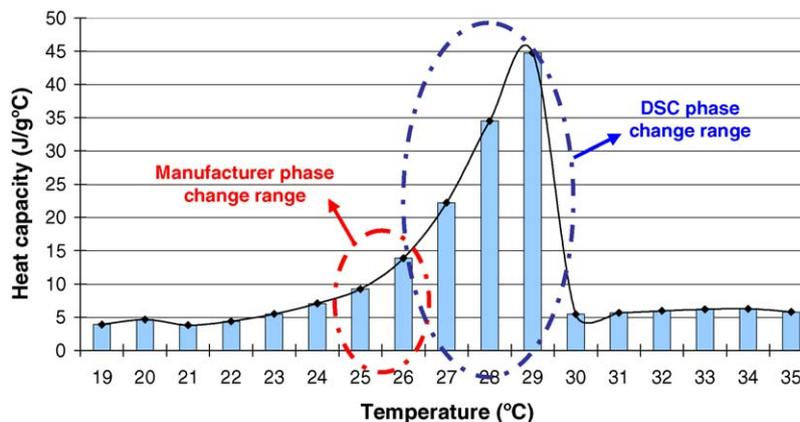
Fig. 12. Specific heat of SP-25 A8. DSC test results.
