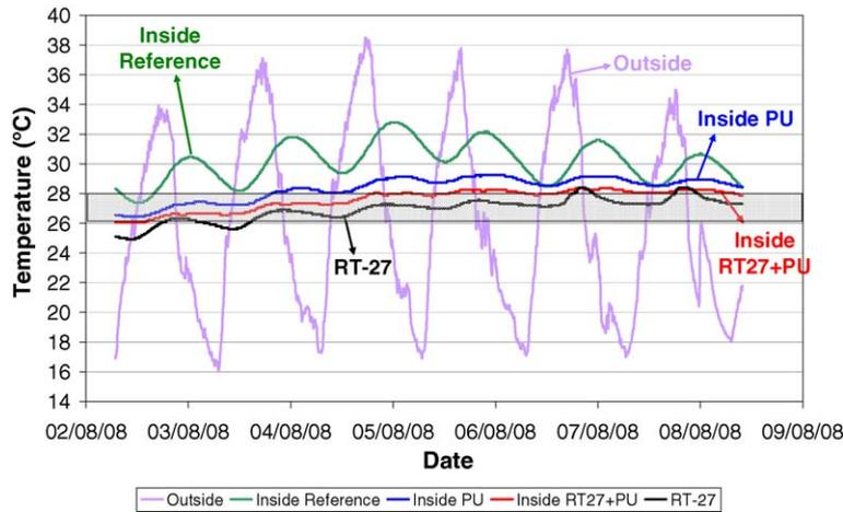
Fig. 13. Conventional brick cubicles. Outside, Inside Reference, PU and RT27 + PU, and RT-27 temperatures.
