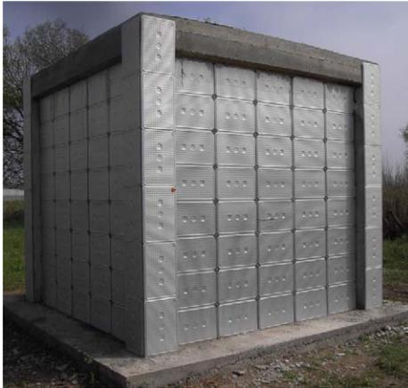
Fig. 6. Brick cubicle with RT-27 and polyurethane.
