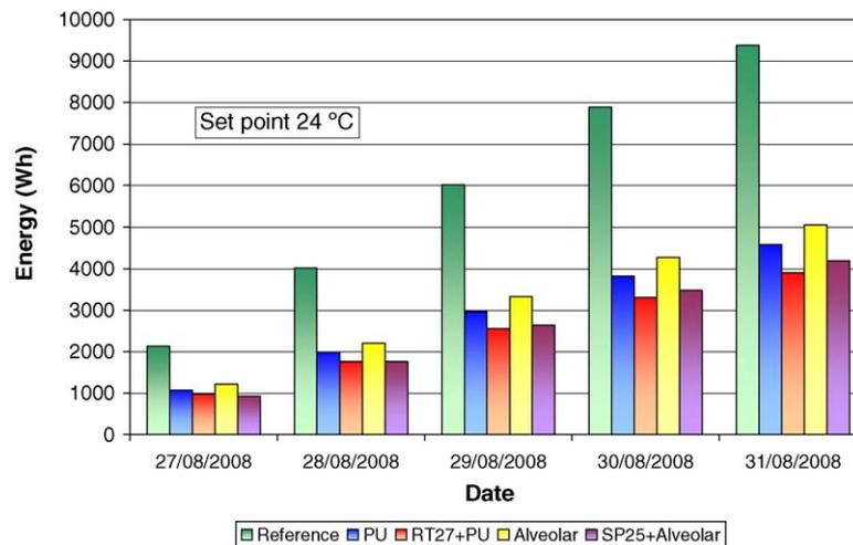
Fig. 17. Accumulated energy consumption. Set point 24 °C.
