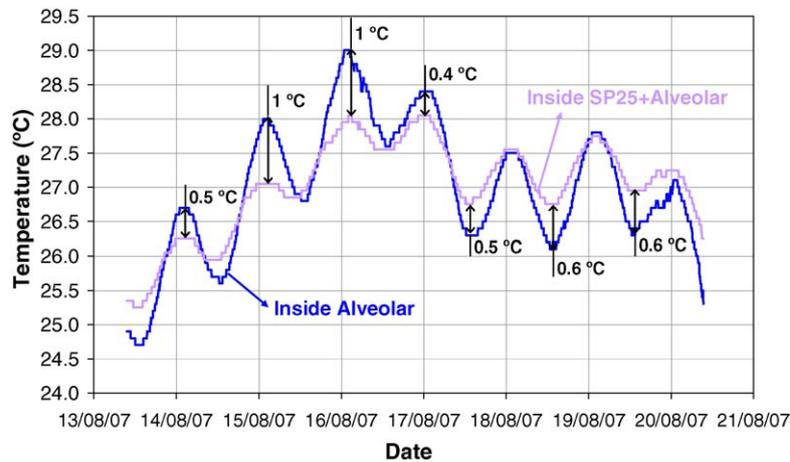
Fig. 16. Alveolar brick cubicles. Inside Alveolar and SP25 + Alveolar temperatures.
