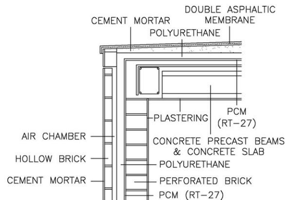
Fig. 9. Section of the constructive solution for the brick cubicles.
