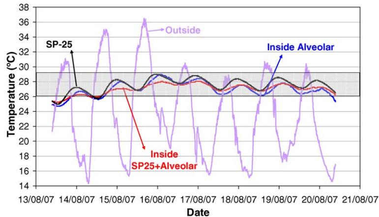
Fig. 15. Alveolar brick cubicles. Outside, Inside Alveolar and SP25 + Alveolar, and SP-25 temperatures.
