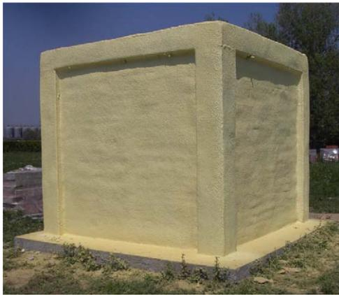
Fig. 5. Brick cubicle with polyurethane.
