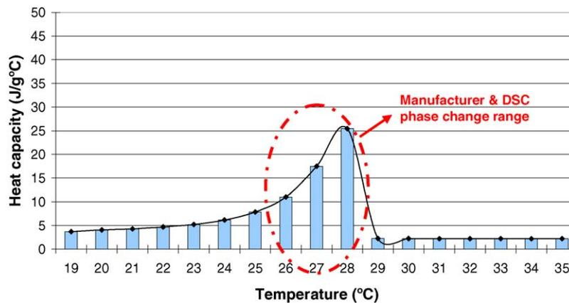
Fig. 11. Specific heat of RT-27. DSC test results.
