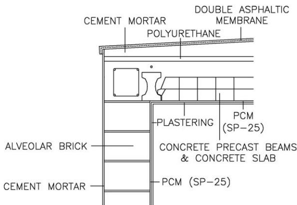
Fig. 10. Section of the constructive solution for the alveolar brick cubicles.
