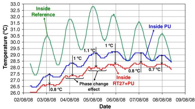
Fig. 14. Conventional brick cubicles. Inside Reference, PU and RT27 + PU temperatures.
