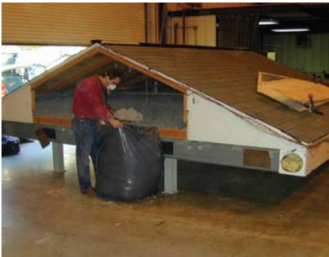
Figure 6. Test attic module used for testing of PCM-enhanced cellulose.
